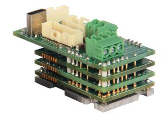
The **FM060-5-EM** is a single-axis servo drive and integration board assembly for a FE060-5-EM FlexPro<sup>®</sup> series servo drive with IMPACT<sup>TM</sup> architecture. Connections to the controller, motor, power, and feedback are simplified through the standard connectors featured on the board.
