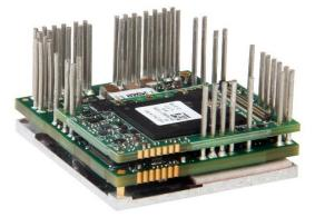
The **FE100-50-CM** is a FlexPro<sup>®</sup> series servo drive with IMPACT<sup>™</sup> architecture.
