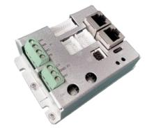
The **CFD060-5-EM** offers full tuning control of all servo loops and is designed to drive brushed and brushless servo motors, and closed loop stepper motors. The drive assembly accepts a variety of external command signals, or can use the builtin Motion Engine, an internal motion controller used with Sequencing and Indexing commands. Programmable digital and analog I/O are included to enhance interfacing with external controllers and devices.
