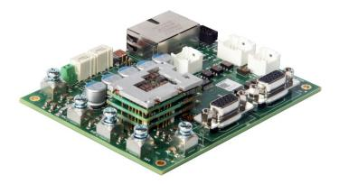
The **FD060-10-EM** is a serve drive and development board assembly for a FE060-10-EM FlexPro<sup>®</sup> series serve drive with IMPACT<sup>™</sup> architecture. Connections to the controller, motor, power, and feedback are simplified through the standard connectors featured on the board. The **FD060-10-EM** is ideal for prototyping and can be used in production and industrial environments as well.
