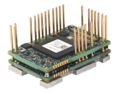
The **FE060-25-CM** is a FlexPro<sup>®</sup> series servo drive with IMPACT™ architecture.
