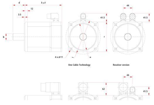
Deviating motor connection for AM8563-wTyz
