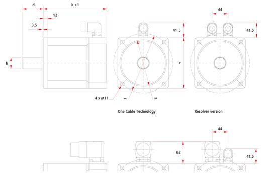
Deviating motor connection for AM8563-wTyz
